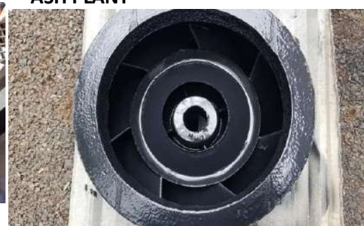
CERAMIC COATING APPLIED ON INNER SUFACE OF OPHERS OF ASH PLANT
