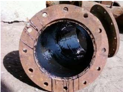
INNER CERAMIC COATING ON T-BEND COATING ON VENTURY OF BOILERS SEA WATER PIPE
