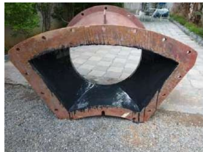
CERAMIC COATING APPLIED ON INNER SUFACE OF OPHERS OF ASH PLANT
